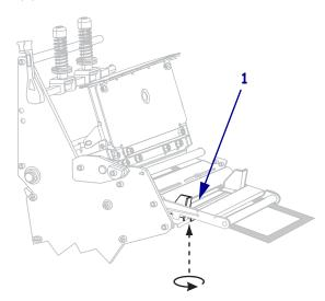
**17.** Push down the printhead assembly (1), and then rotate the printhead-open lever (2) clockwise until it locks into place.
